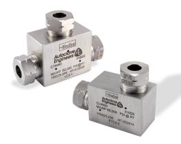
Parker Autoclave Engineers High Pressure Cone & Thread Fittings, Couplings, Filters and Valves utilize the F Style Cone & Thread Connection Detail (see Tools & Installation brochure for dimensions). These fittings are compatible with Series 30SC, 43SC, 30VM, 40VM, and 60VM valves and Parker Autoclave Engineers high pressure tubing.
