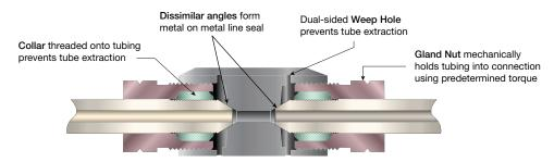
High Pressure design "encapsulates" collar keeping connection depth to minimum
