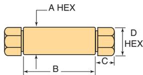
**Note:** Union Couplings are designed with a removable seat insert allowing disassembly and tubing removal without the necessity of loosening other items in a line.
