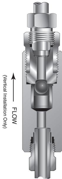
Protects pressure gauges and pressure instrumentation from sudden surges in flow or venting in the event of line failure.
