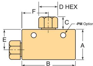
**Note:** Fittings such as 45° elbows, reducer elbows, and reducer 45° elbows are available upon request. For mounting hole option add suffix - **PM** to catalog number, consult factory for mounting hole dimensions.
