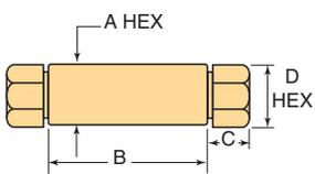
**Note:** Union Couplings are designed with a removable seat insert allowing disassembly and tubing removal without the necessity of loosening other items in a line.
